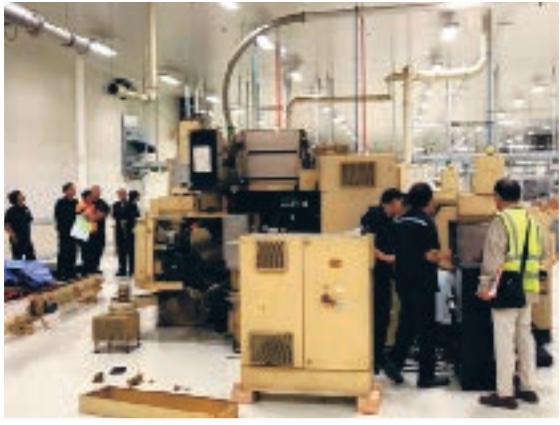
Relocation of old machine from Khlong Toei to Ayutthaya, Installation of rolling machine Protos70 No.15 and packaging machine Alfa Ram No.24 being installed at TOAT Ayutthaya
